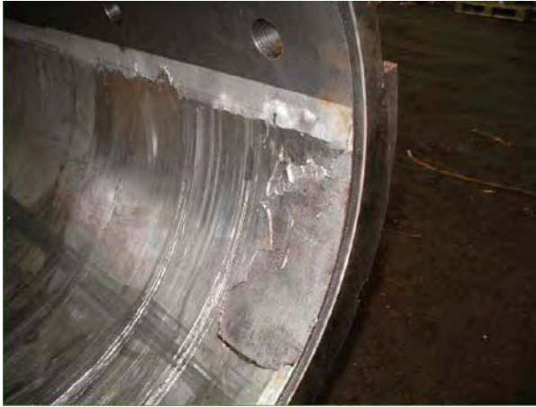
Fig. 1.6 Fatigue damage of the stern tube bearing [3]
