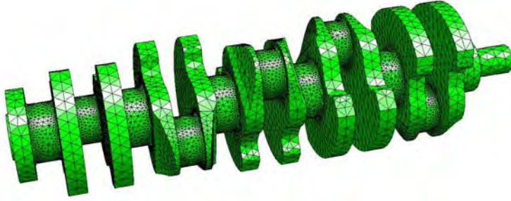
Fig.5.5 Crankshaft 3-D solid model
