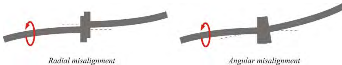
Fig.4.7 Propulsion shafting alignment errors
