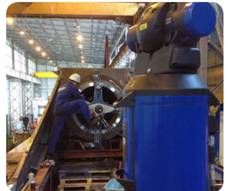
3D measurement in combination with on-site machining
