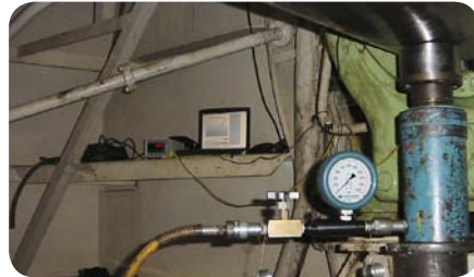
Load cell and hydraulic jack near shaft bearing
