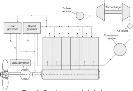
Figure 5 – Propulsion plant principal scheme
