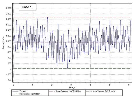
Figure 4 – Torque in the propeller shaft
