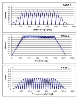
Figure 1 – Ice induced torque graphs
