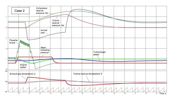
Figure 6 – "Snow Dragon" propulsion plant dynamics parameters
