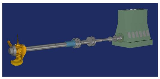
Figure 2 – Propulsion shafting model of "Snow Dragon" ship
